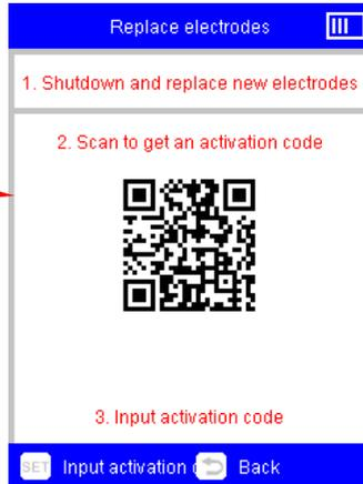
the splicer and replace by new and original COMWAY electrodes (ID electrode).
