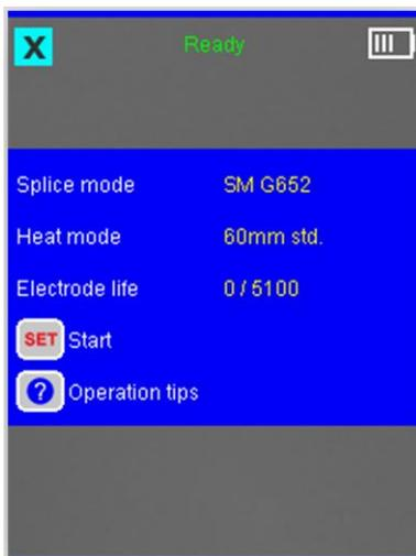
6. After finishing all steps of electrode replacement , please enter into the “Maintenance menu” to implement “Electrode stabilize” and “ARC adjust
