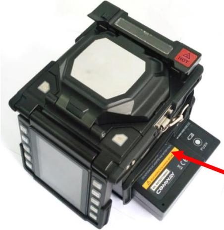
Insert the [Battery Pack](#) into the machine in the direction as indicated by the red arrow.
