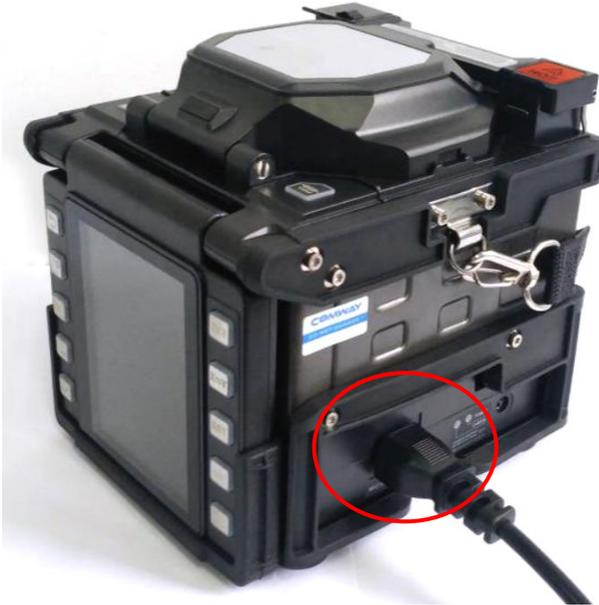
1. Remove the [Battery](#) from the machine;
