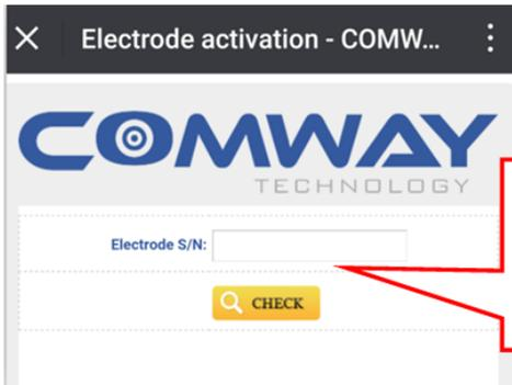
Input the serial number in the original COMWAY electrode (ID electrode) package and press "CHECK".
