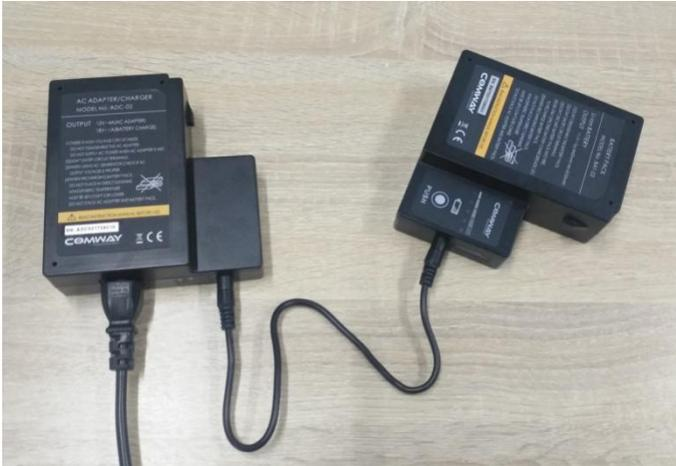
1. Connect the AC Adapter with the Battery by [DC Power Cable](#);
