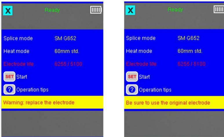
3. When the electrodes' used times reach to or over the total lifetime, there will be scrolling notices, as shown above.
