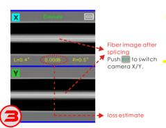
Loss is estimated and displayed after splicing finished.
